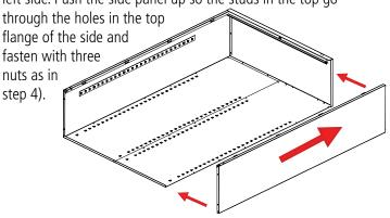
**6.** Attach the sill (Ref. No. 8) to the sides. Place nuts loosely on each of the studs and slide the ends of the sill into the slots on both sides of the unit. Then, securely tighten the nuts.
