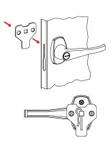
With the handle still in the open position, hook the locking bars (Ref. No. 9) to the locking cam (see "A" at left). Once in position, slowly rotate the door handle to the closed position so the lock bars prot rude from the holes at the top and bottom of the door (shown at right, below).
